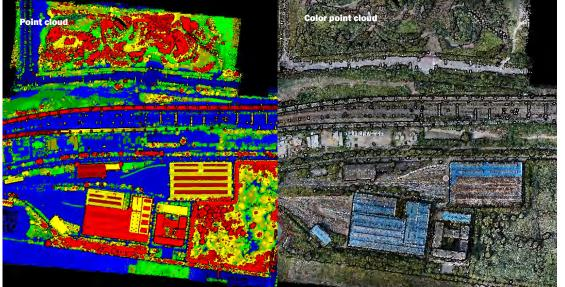
Model:GS-260X Flight speed:10m/s Flight altitude:120m Accuracy:5cm Application:Track Monitoring Project location:China
